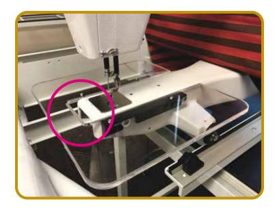
Push the ruler base back until it is touching the machine or snaps into place.
