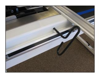
10. With the power cable unplugged and the motors in the engaged position (use the manual engagement/disengagement tool if necessary), ensure that as the quilting machine is moved in both the X and the Y directions, the corresponding gears are rotating as well.
