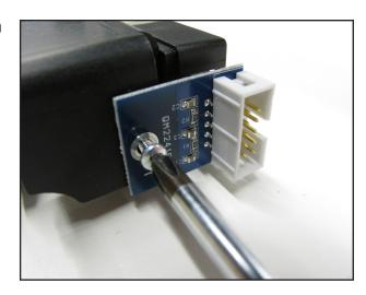
3. Gently pull the circuit board outward toward the front of the quilting machine (the same direction the screw came out).
