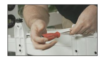
8. Attach the Y-Rack to the bottom of the front and rear base plates. The blue Flexirack should be toward the middle of the machine while the bolt holes should be toward the outside. Use the screws that were removed from the front and rear base plates (or use the two smallest screws in the Base Plate Repair Kit [see Parts List, item D] if your machine had no screws here).
