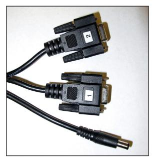
Insert the barrel connector into the center jack located on the bottom edge of the black box that is mounted to the back of the computer bracket. Attach the two 9-pin serial cables to the appropriate ports on the back of the same box, making sure cable connectors are plugged into their corresponding ports on the black box.
