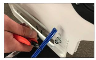
6. At both ends of the blue Flexirack, use two of the small metal clamps (see Parts List, item B) to hold the ends firmly in place. The clamps have a hole through the center and a lip on one end. The lip should be on the side opposite the blue Flexirack. Place the clamps where they will be attached and drill pilot holes using the 3/32-inch drill bit and then use a Phillips screwdriver to fasten the clamps on both sides of the Flexirack to the table.
