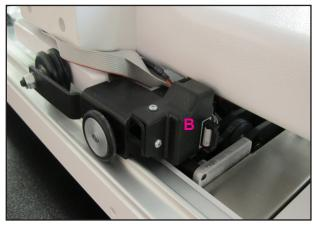
3. Attach one end of the harness cable (see Parts List, item P) into the connector on the right side of the power supply. Tighten the side screws. You will plug the other ends to the bracket as part of step 5 when you attach the tablet computer.
