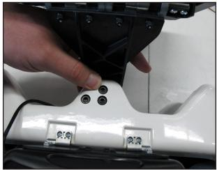
4. Secure the handlebar and bracket in place on the machine head using the three handlebar bolts.
