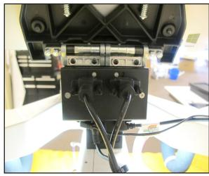
Remove the computer from its packaging. Lift up slightly on the center of the top bracket and install the computer into the computer bracket by sliding it into the black bracket from the side until it is centered.
