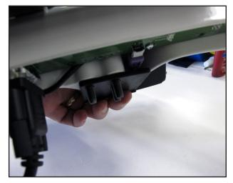
3. Position the handlebar over the computer bracket such that the screws go through the three holes in the bracket.
