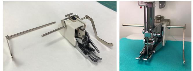
1. Place U-Shaped piece over the top of foot and line up with the holes on the foot.
