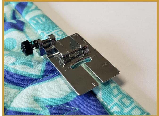
4. The inside edge of the deeper side of the foot should rest right next to the inside edge of the binding allowing the foot to rest flat on the project.
