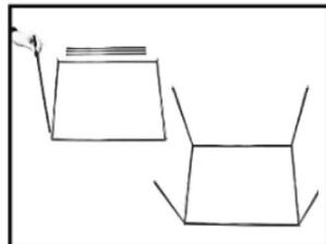
4. Complete assembly by adding the remaining assembled frame to the side rails, again inserting the pegs at each corner into the side rails.
