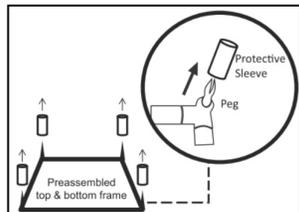
3. Insert the four side rails onto the pegs at the corner of each side of one assembled frame.
