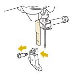
4. Set the adapter on the presser foot bar, aligning the flat side of the adapter opening with the flat side of the presser bar. Push it up as far as possible, and then tighten the screw securely with the disc-shaped screwdriver.
