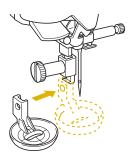
Tighten the screw with the included screwdriver (large).
