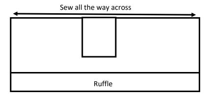
Set your machine for 3-thread overlock narrow stitch with decorative thread in the upper looper and lower looper (Madeira Decora 12-weight contrasting or complimentary), regular serger thread in needle. Set the stitch length at 1, stitch width at 4.0 and make sure the knife is in an engaged and cutting position.
