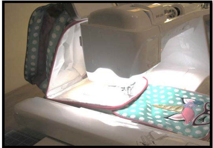
This image shows the bulk of the lunchbox behind the machine head. You can see, I still need to move the needle so it doesn't stitch on the inner lunchbox! I had to bring the hoop in from the back side to get it under the needle and then to slide into the machine.
