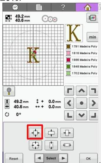
13. Center the letter over the center mark on the bag by using the arrow keys on the screen to move the letter, while using the needle beam as your guide.
