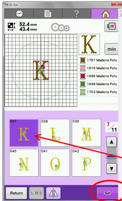
12. To resize the letter smaller, click on the Size icon. Click on the first icon with the arrows pointing inward until the size of the letter is less than 50mm as shown in the following illustration. The size in the sample was 49.2mm. On this machine you can resize downward 10% and upward 20%.
