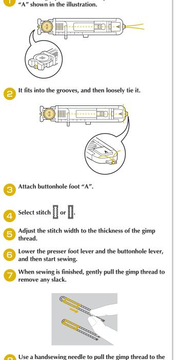
Hook the gimp thread onto the part of buttonhole foot
