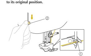
Lower the needle threader lever on the left side of the
