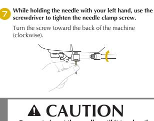
• Be sure to insert the needle until it touches the needle stopper and securely tighten the needle clamp screw with the screwdriver, otherwise the needle may break or damage may result.
