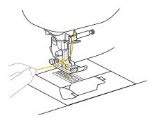
6 Pull up the bobbin thread, pass it under the presser foot and pull it about 10 cm (4 inches) toward the back of the machine, making it even with the upper thread.
