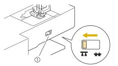
Feed dog position switch (as seen from the rear of the machine)
