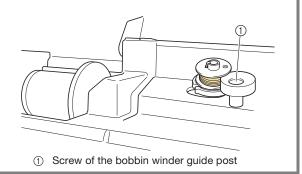
If the thread become tangled under the bobbin winder seat, press the "Start/Stop" button once to stop the bobbin winding.
