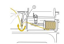
Pass the thread under the thread guide plate, and then
