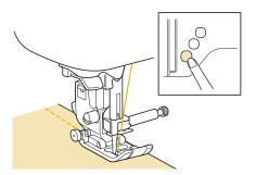
$\bigcirc$  Press the  $\Join$  (Thread cutter button) to trim the upper and lower threads.
