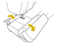
A presser foot accessory tray is stored in the accessory compartment of the flat bed attachment.
