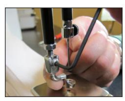
NOTE: We recommend that you use the 1.5mm couching foot to ensure the foot is centered with the needle. Then slowly rotate the hand wheel to confirm its position and check the other couching feet position.
