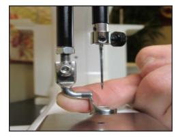
3. Ensure the foot is centered with the needle when the foot is fully tightened with the 2.5mm hex wrench. If it isn't properly centered, loosen the lock nut; center the foot with the needle; hold the foot in position; and firmly tighten the lock nut. Recheck the position.
