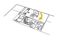
5 Insert the tabs on the needle plate cover into the needle plate, and then slide the cover back on.
