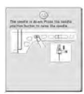
This message is displayed when the embroidery unit is attached and the power is turned on with the needle in the down position.
