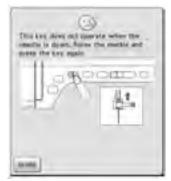
This message is displayed when a key on the LCD display is touched while the needle is in the down position.
