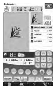
→ When the last color is sewn, "Finished sewing" will appear on the display. Press \_\_\_\_\_, and the display will return to the original screen.
