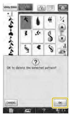
→ The machine deletes the stitch pattern, then automatically saves the new stitch pattern.
