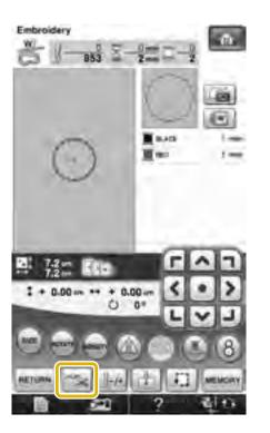
Press E to turn off the thread trimming function.
