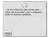
This message is displayed when the foot controller is pressed while the embroidery unit is attached and machine is set up for embroidering.
