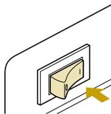
► The sewing lamp and the LCD come on when the machine is turned on.
