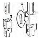
4. **Note:** When attaching the adapter, be sure to use a screw driver to tighten the \*small screw firmly.
