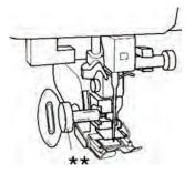
**Note:** Before sewing, be sure to turn the handwheel toward you slowly to check that the foot is attached properly and the needle does not touch the presser foot.
