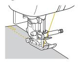
When the end of the stitching is reached, press ("Reverse/Reinforcement Stitch" button).
