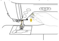
If thick seams are being sewn and the fabric does not feed at the beginning of stitching Zigzag foot "J" is equipped with a feature that keeps the presser foot level.
