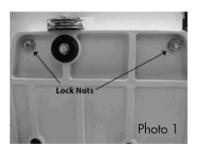
for locating and holding the carriage bolt head during tightening). Attach with the two lock nuts on the bottom of the machine's base plate (See Photo 1) and tighten until the bracket is firm and does not move. Lift the machine upright and place back on the carriage for the next step.
