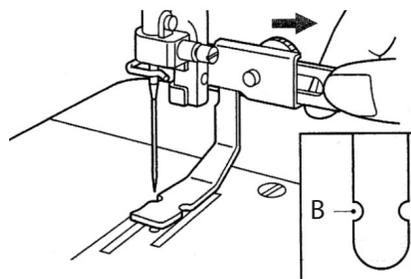
11. Turn the handwheel to lower the needle, position the presser foot and tighten the adjustment screw before sewing.
