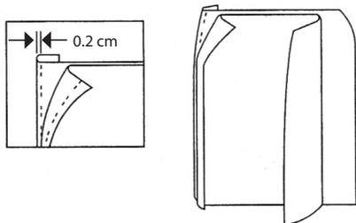
7. Secure the zipper with basting and sew along the mark.
