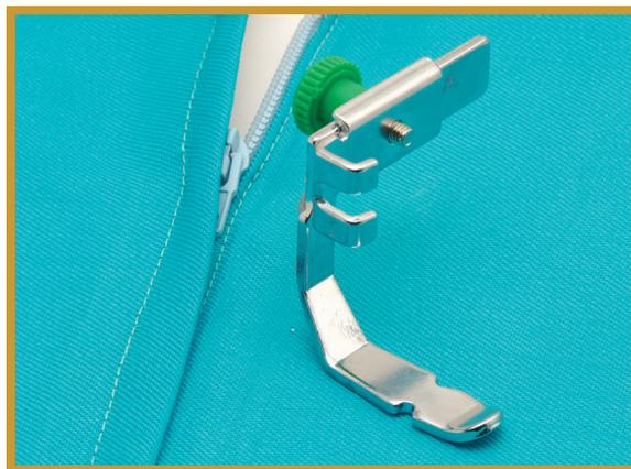
10. Loosen the zipper foot screw to change the position of the zipper foot.
