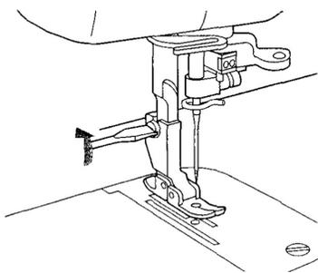
3. Attach the zipper foot and tighten the screw.
