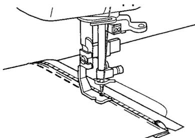
**NOTE:** Make sure the needle does not strike the metal part of the zipper when sewing. The needle may break and cause injury.
