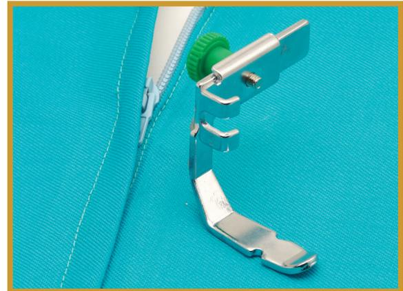
4. Turn the handwheel toward you to lower the needle. Adjust the position of the foot relative to the needle using the adjustment screw to slide the foot from left to right. Then tighten the zipper foot adjustment screw.
