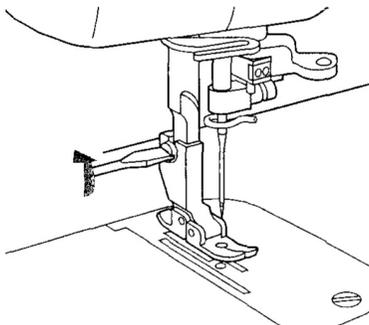
3. Attach the 8mm Bi-level Spring Action Guide foot and tighten the screw.
