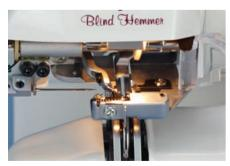
Needle & Lighting Area Uses standard, easy-to-insert household needles in a workspace illuminated with a built-in light
