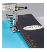
**Note:** The lower portion of the ruler can flex to curve around the bed of the sewing machine depending on the model.
