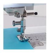
Remove the clear backing and set seam guide against right side of foot. The seam guide has recessed areas on the lower side so that it sits directly over the right feed dog of the machine and over the 1/4 inch mark of the clear bobbin cover.
