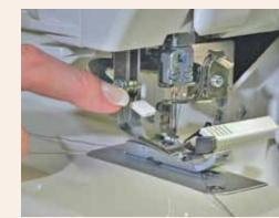
Baby Lock has put a lot of thought into threading a serger including the most important part—the needles. Baby Lock's easy-to-use needle threader remains fixed as you easily thread the needles with the touch
