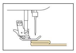
**Note:** Once the trouble spot has been passed, the foot will return to its normal position. When "Automatic Fabric Sensor System" (Automatic Presser Foot Pressure) in the machine settings screen is set to "ON", the thickness of the fabric is automatically detected by the internal sensor so the fabric can be fed smoothly for best sewing results.
