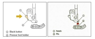
5. Place the new presser foot under the holder, aligning the foot pin with the notch in the holder. Lower the presser foot lever so that the presser foot pin snaps into the notch in the holder.
