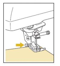
3. Release the black button. The presser foot remains level, enabling the fabric to be fed.
