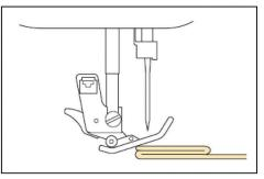
If the presser foot is in the up position, and you are sewing heavyweight or multiple layers of fabric which do not fit easily under the presser foot, use the presser foot lever to raise the presser foot to its highest position. The fabric will now fit under the presser foot.
