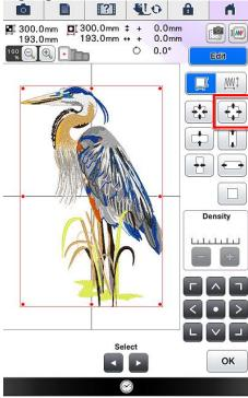
• Click on the sizing tool that is inside the red box (as shown in the illustration above) ten times. This tool will increase the size of the design 20%, its largest size, while creating a less dense design. The stitch count on the design will be the same as on the original design. This will reduce the density level on the design which will work very well when embroidering over the layers on the pieced section.
